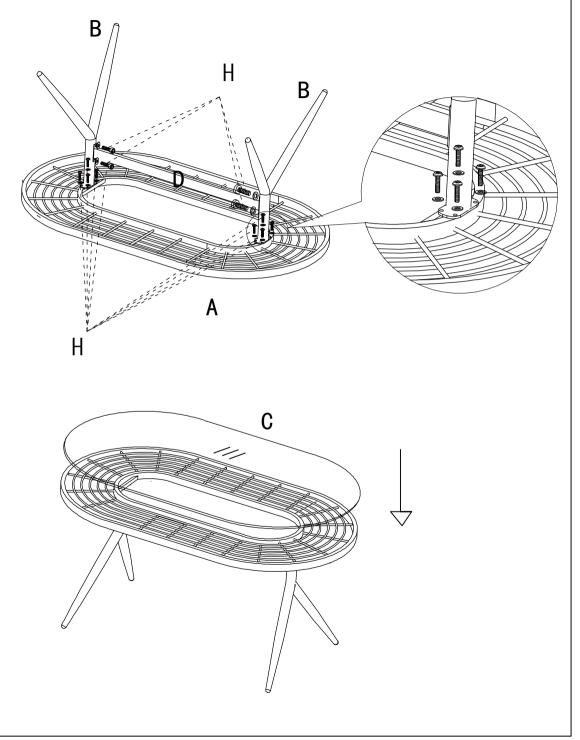
Do not fully tighten bolts until assembly is complete.
